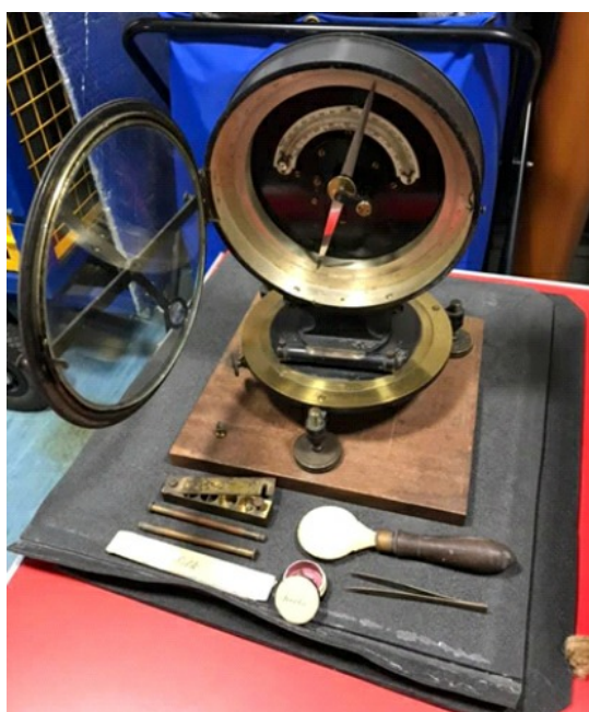
The Fox dipping needle, and Dr Edward Gillin demonstrating it at the Fox Cafe, Falmouth University. Photos: Edward Gillin and Mary Hesling
